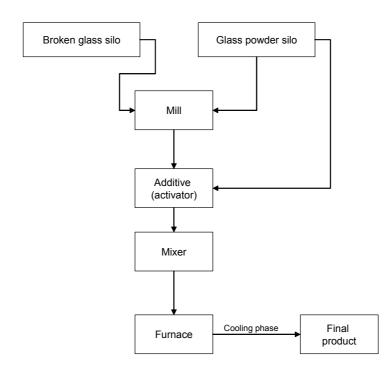
Figure 34: The Foam Glass Production Process
