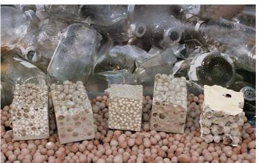
From glass, to pellets to products (Geofil-bubbles)
