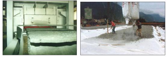
Figures 7 and 8 - Foam glass exiting the furnace and being used for a loose aggregate floor insulation
