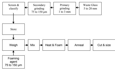
Figure 2 - Process route for foam glass production.
