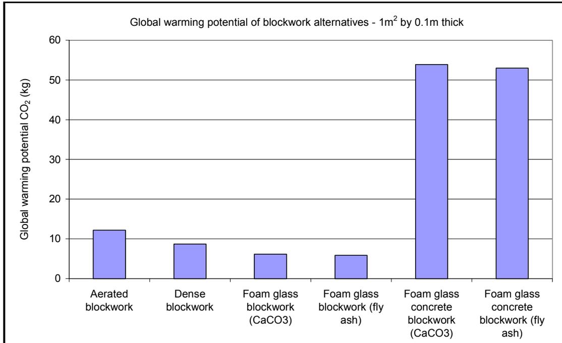
Figure 44 - Global warming potential of blockwork alternatives
