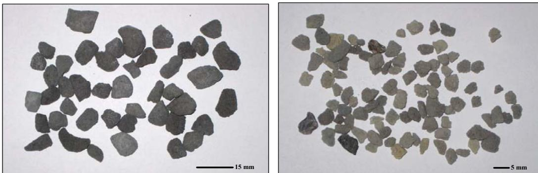
Figure 10 - Medium and Small sized loose aggregate foam glass.
