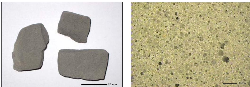
Figure 9 - Misapor's large loose aggregate foam glass and pore structure.
