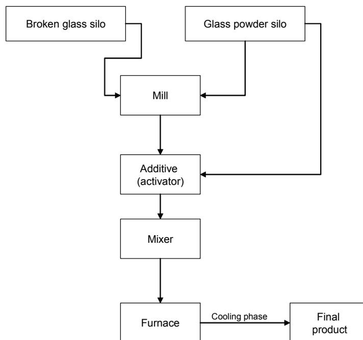
Figure 34: The Foam Glass Production Process
