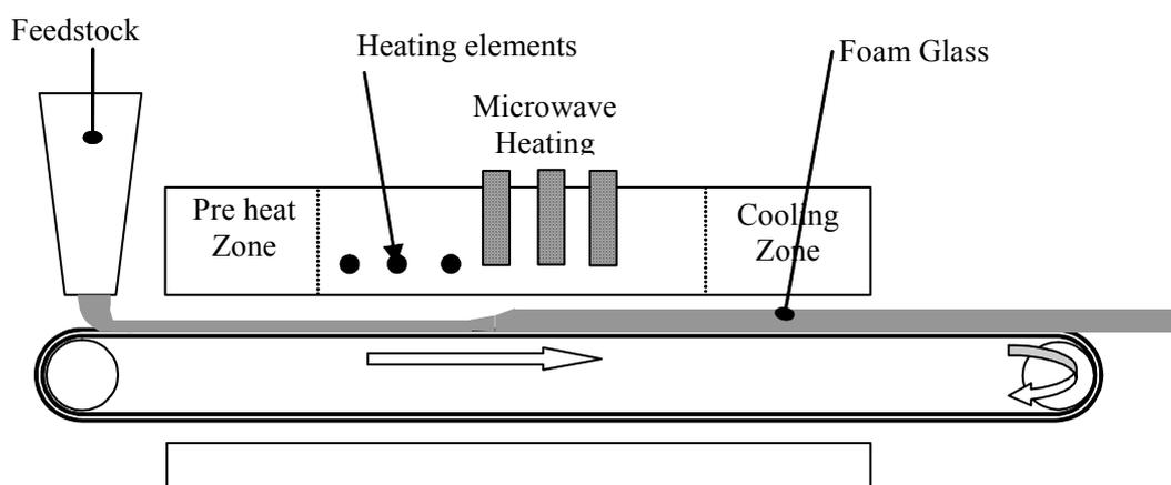
Figure 49 - Continuous furnace for production of foam glass using dual heating, conventional electric and microwave radiation.
