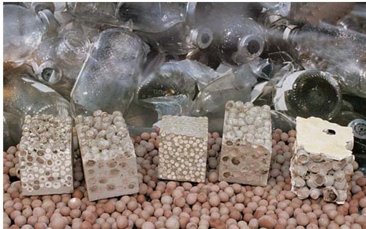
From glass, to pellets to products (Geofil-bubbles)
