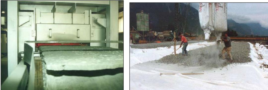
Figures 7 and 8 - Foam glass exiting the furnace and being used for a loose aggregate floor insulation
