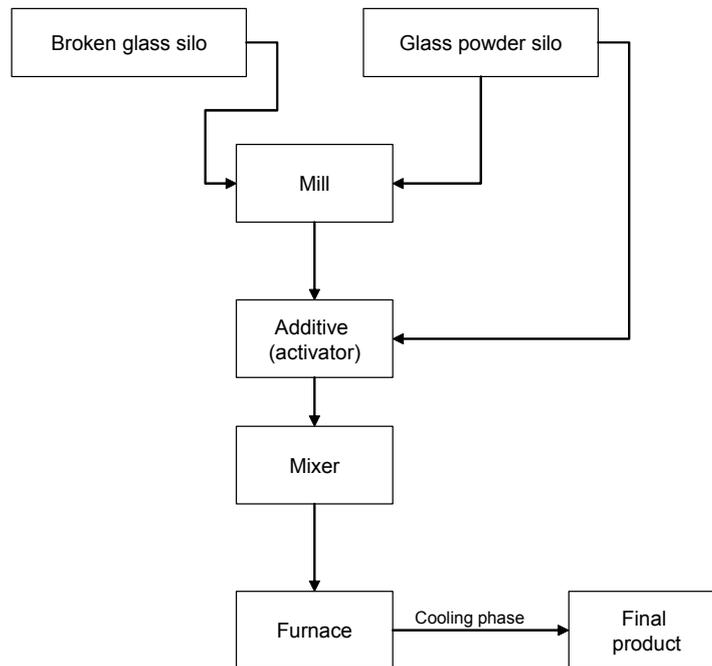
Figure 34: The Foam Glass Production Process
