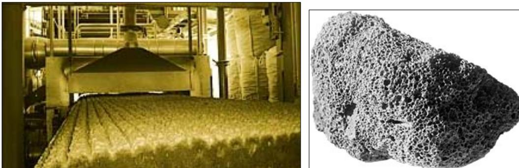
Figures 14 and 15 - Millcell foam glass continuous production and loose aggregate particle<sup>38</sup>
