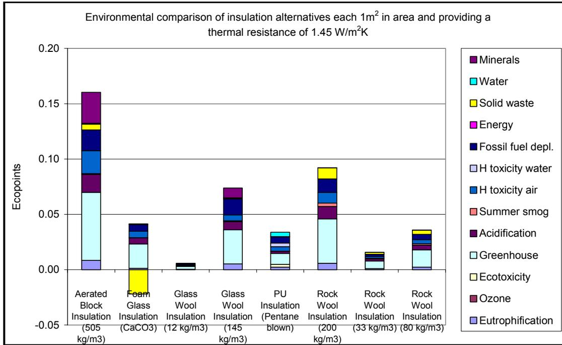
Figure 47 - Environmental Comparison of Insulation Alternatives
