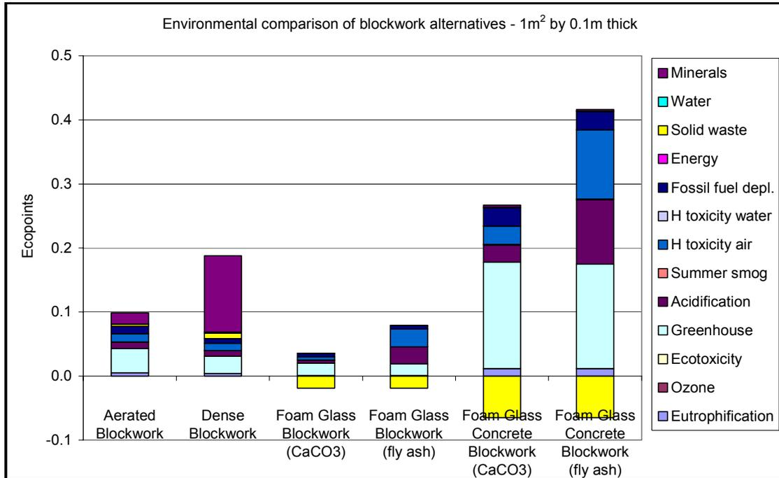
Figure 45 - Environmental comparison of blockwork alternatives
