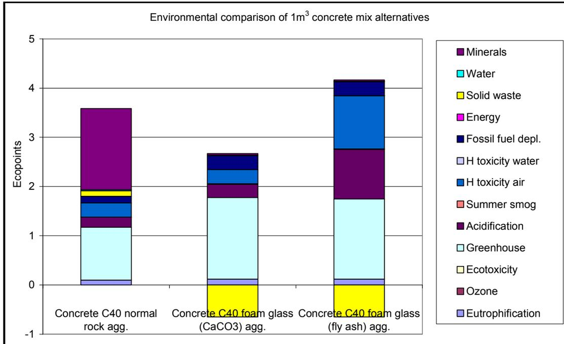
Figure 43 - Environmental comparison of concrete mix alternatives
