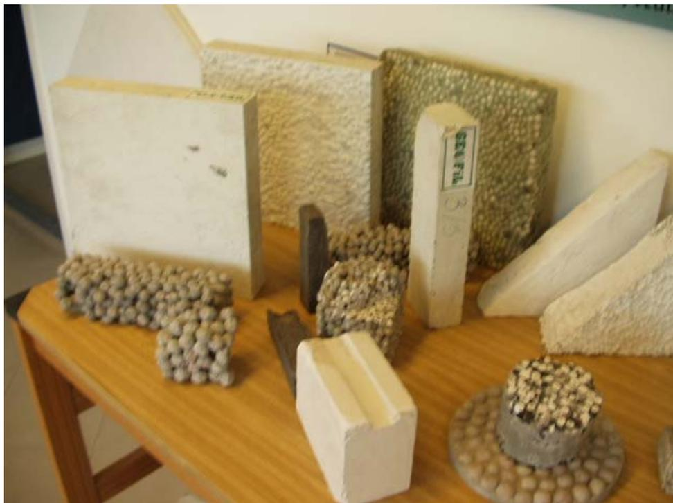
Figure 13 – Various trial products developed by Geofil using Geofil-bubbles.
