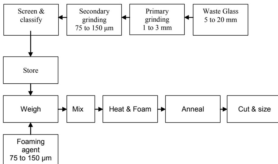
Figure 2 - Process route for foam glass production.
