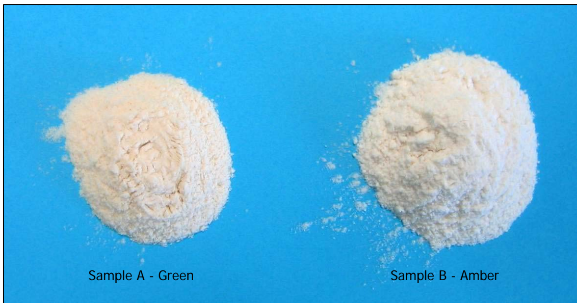
Figure 15 Sands from green (sample A) and amber (sample B) cullet produced by the alkali fusion route.
