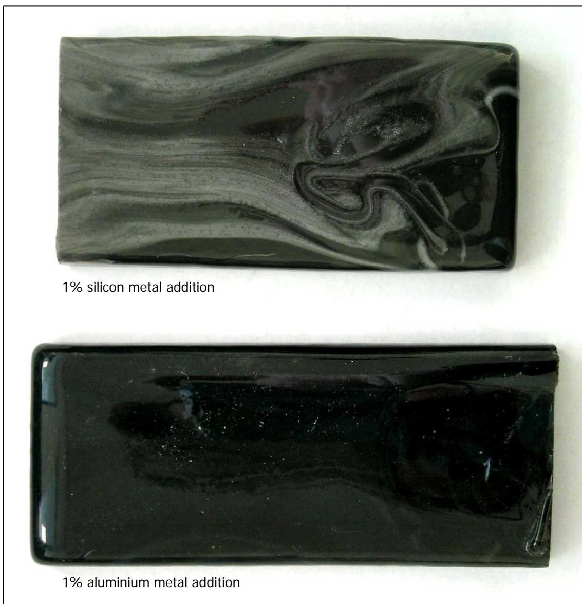
Figure 14 Reductive melting samples with 1% silicon and 1% aluminium fine metal particle additions into the glass melt (green glass).
