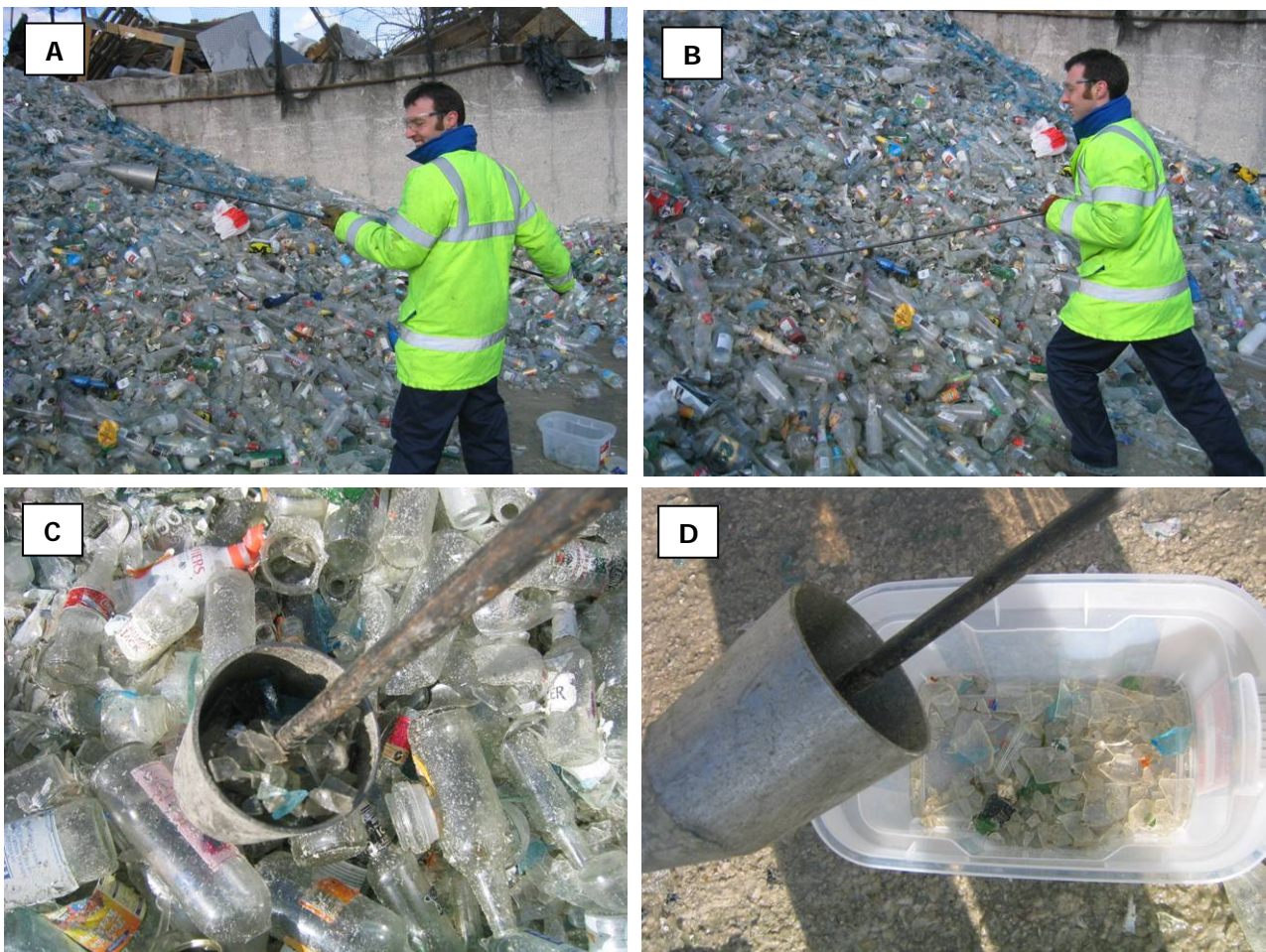
Figure 3 Design and use of a simplified sample thief
