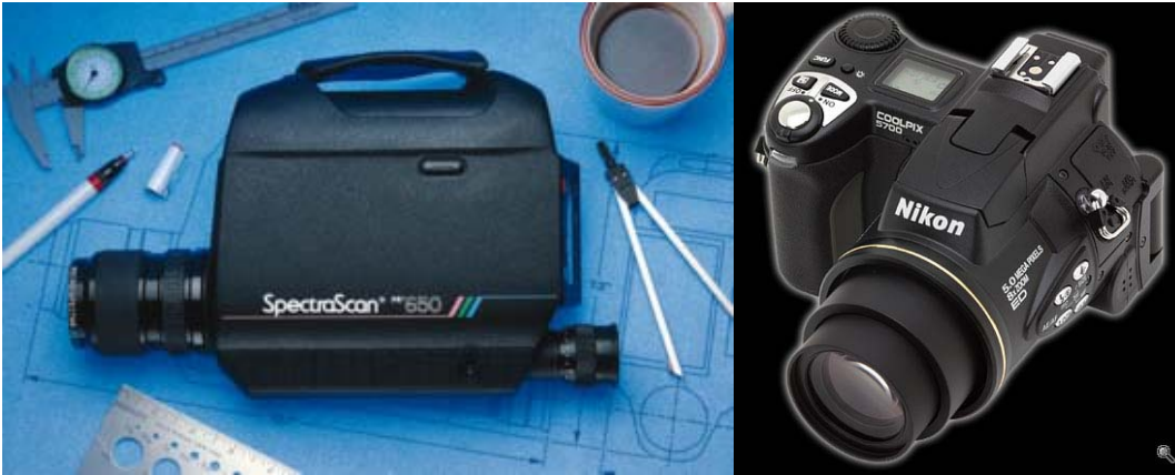
Figure 2: A Photo Research PR-650 tele-spectroradiometer (left) and a Nikon Coolpix 5700 digital camera (right).
