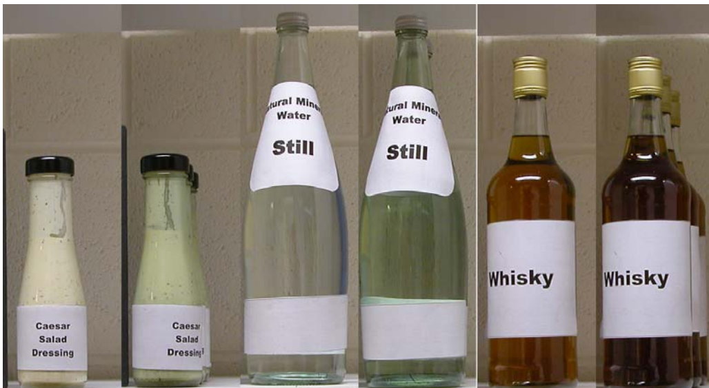
Figure 1: Three kinds of products, each was put into 3 different bottles with slightly different green colours and measured either single or in a row.
