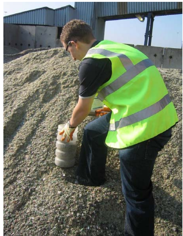
Figure 27: Multiple sampling model from the cullet pile and an operative taking a sample from a cullet pile.
