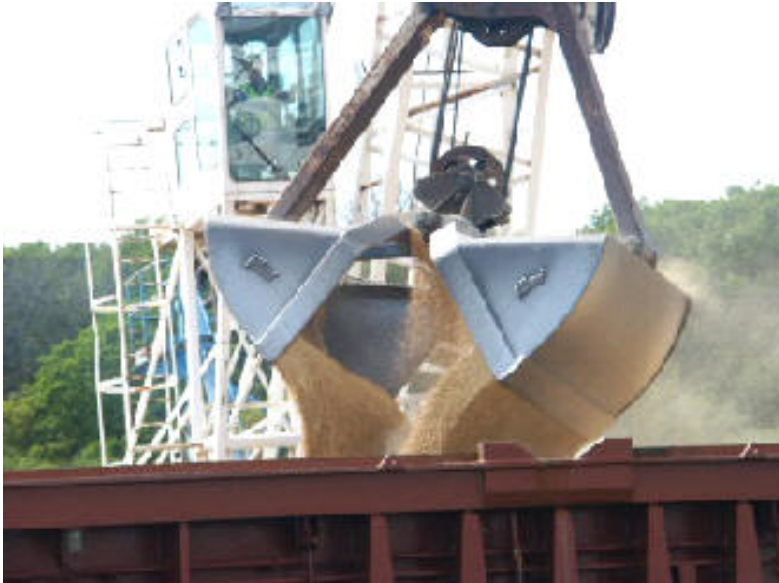
Figure 16. An example of the grab system used to load vessels.
